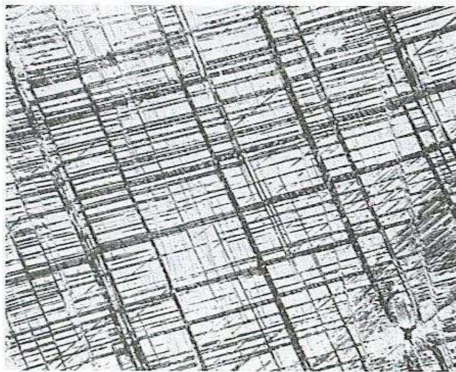
Figure 3-41 Microstructure of explosively hardened Hadfield Mn steel (sheet martensite) revealed using 2% nital followed by 20% aqueous sodium metabisulfite, 375 \times .
