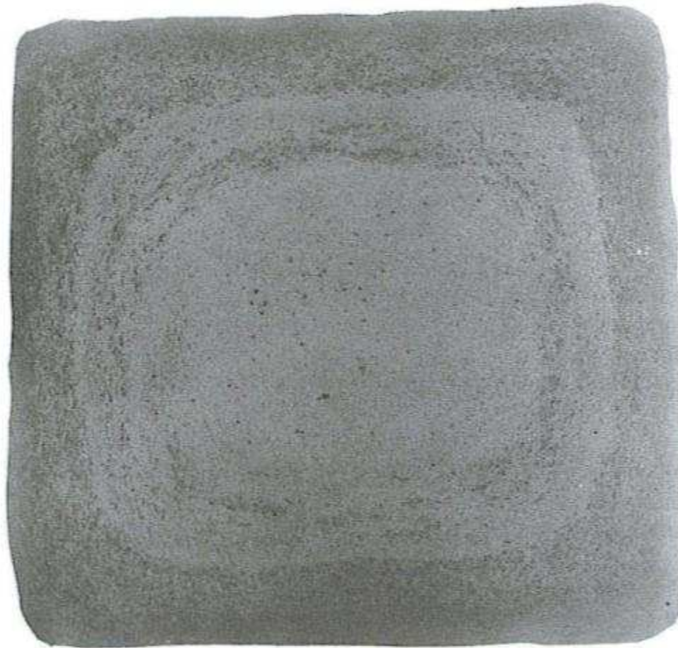
Figure 1-5 Hot-acid etching of this 9-in square disc of AISI 4142 alloy steel revealed ingot pattern and inclusion pits.
