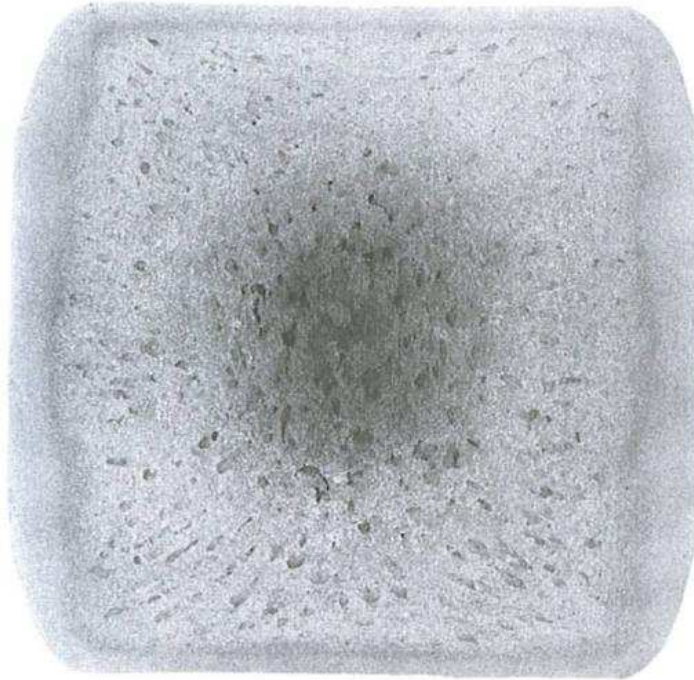
Figure 1-6 Hot-acid etching of this disc from an AISI 4140 alloy steel billet revealed entrapped gas, heavy segregation, voids, and ingot pattern.
