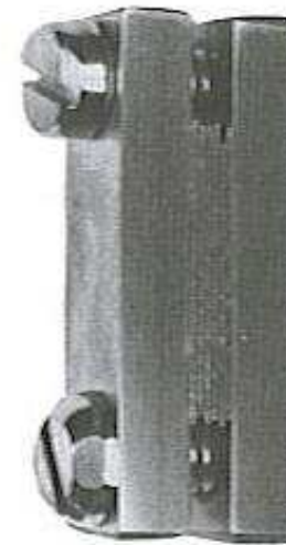
Figure 2-4 Examples of adhesive mounting (left) for planar surface examination and mechanical clamps (right). The clamp has plastic spacers between the specimens.
